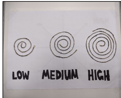
Figure 11. Test board for vibration intensity test.
