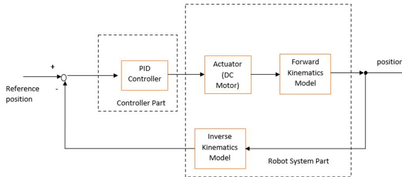
**Figure 4.** The concept of control system for robotic joint display
