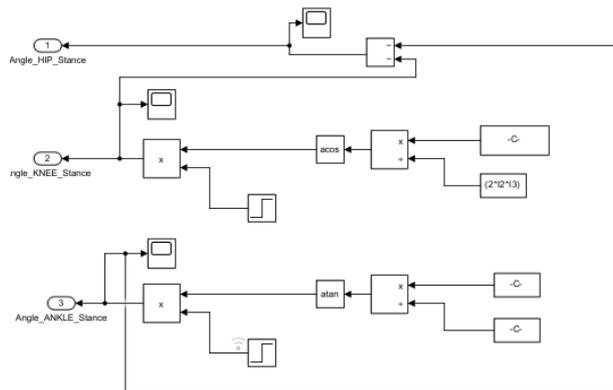
**Figure 3.** Inverse Kinematic Equation of Stance Leg
