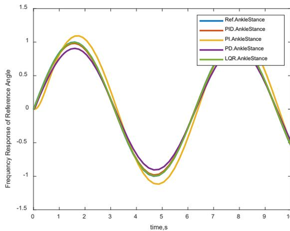
**Figure 9.** Sinewave response of Ankle Joint of Stance Leg
