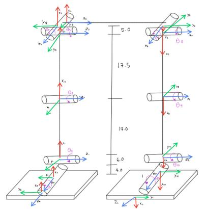
Figure 2. Coordinates frames of Biped Humanoid Robot for each leg joint
