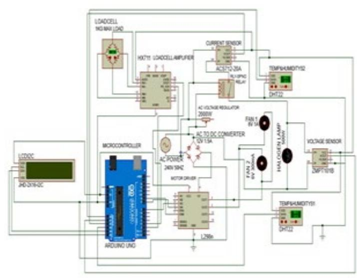
Figure 2. Schematic Circuit of dryer
