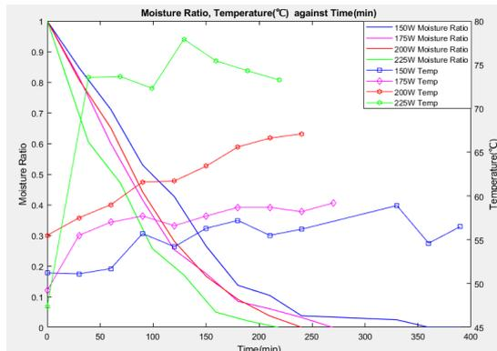
Figure 7. The last 4 parameters graph Moisture Ratio, Temperature against Time (min)
