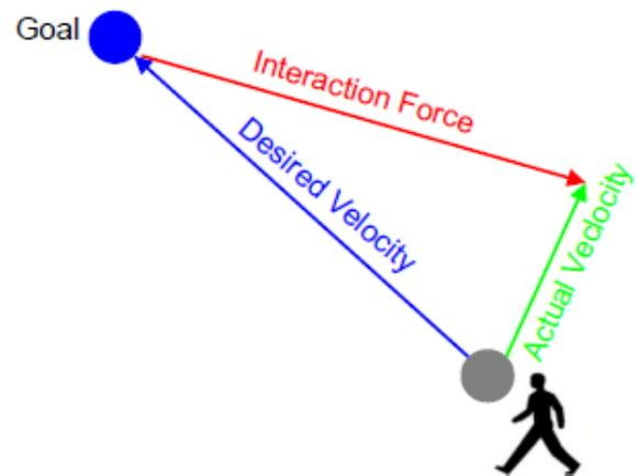
**Figure 1.** Visualization of force and velocities in SFM [44].
