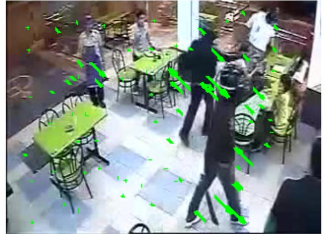
**Figure 5.** Interaction forces computed using SFM.
