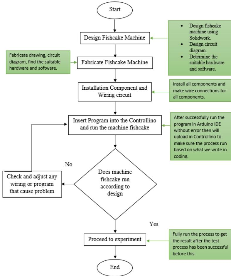
Figure 7. Flow chart for machine fishcake design
