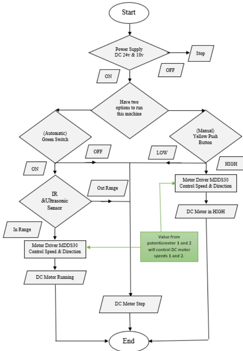
Figure 8. Flow chart for control input and output in Fishcake Machine
