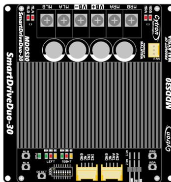
Figure 2. Motor driver type of MDDS30
