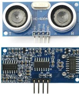
Figure 6. Ultrasonic Sensors type of HC-SR04
