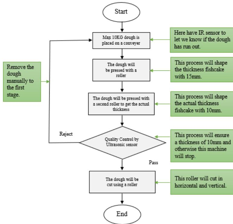
Figure 9. Flowchart to produce fishcake
