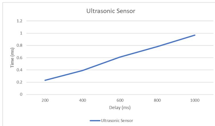
**Figure 11.** Graph action time for the ultrasonic sensor
