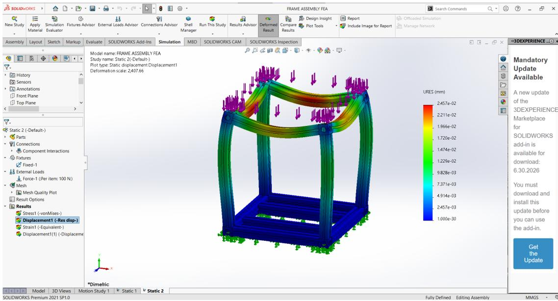
Figure 7 Displacement Analysis
