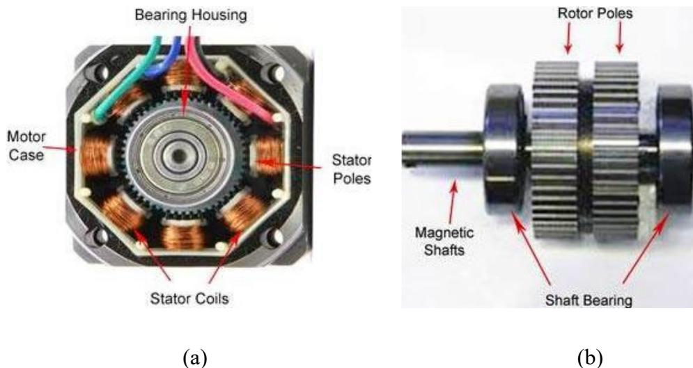
**Figure 1 (a)** Cross Sectional View of a Stepper Motor **(b)** Rotor of a Stepper Motor
