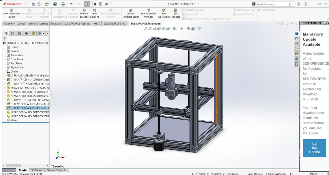
Figure 5 Concrete 3D Printer Design
