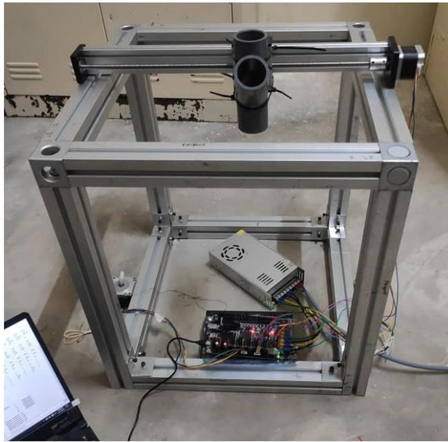
**Figure 10** Concrete 3D Printer Assembly & Testing
