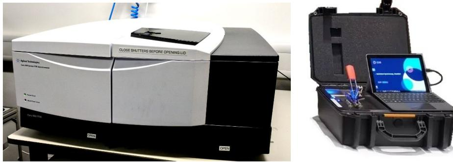
**Figure 1.** Spectrometers utilized in this study: Agilent Cary 660 (left) and BP-10 (Right) .
