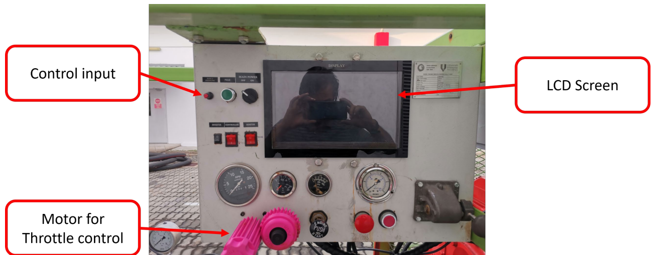
Figure 2. The Control panel used for the system
