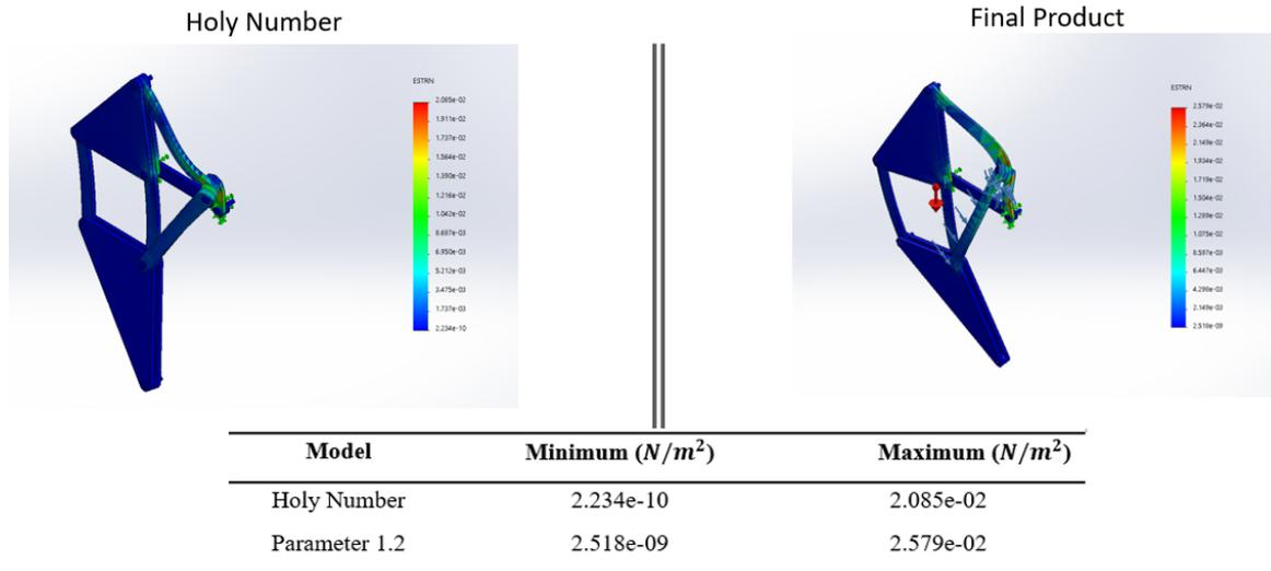
Figure 3. Equivalent Strain Results on Both Model
