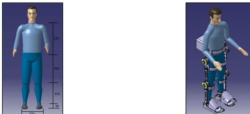
**Figure 9.** (Left) Reference Manikin Body Dimension in mm, (Right) Manikin wearing the proposed exo-suit.
