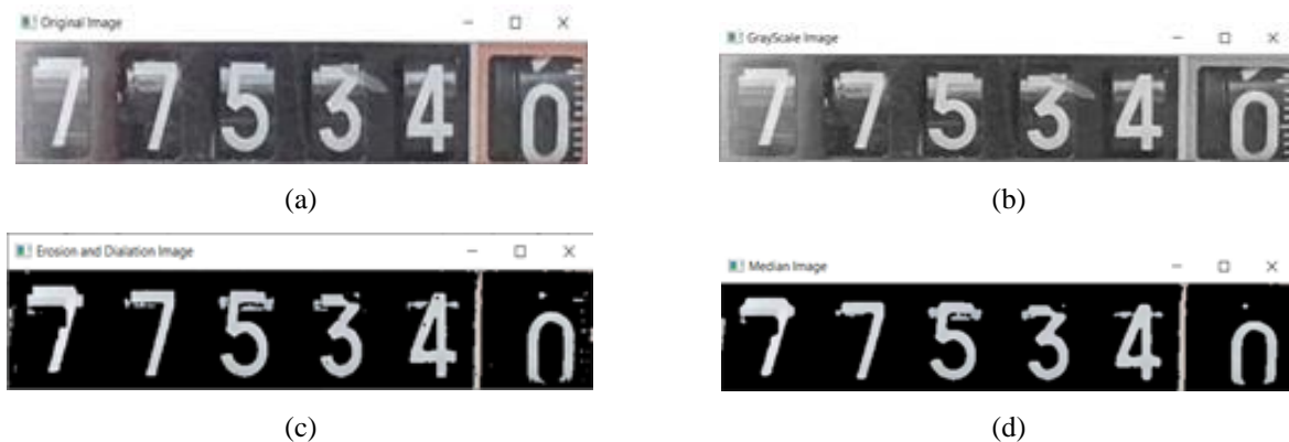
Figure 4. Preprocessing of (a) Original Image, (b) Grayscale Image, (c) Binarized, Erosion and Dilation Image, (d) Median Filtered Image
