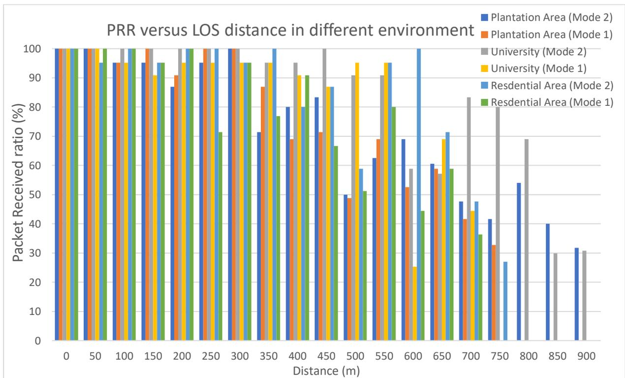
**Figure 10.** The graph for PRR versus LOS distance sensors in different environments
