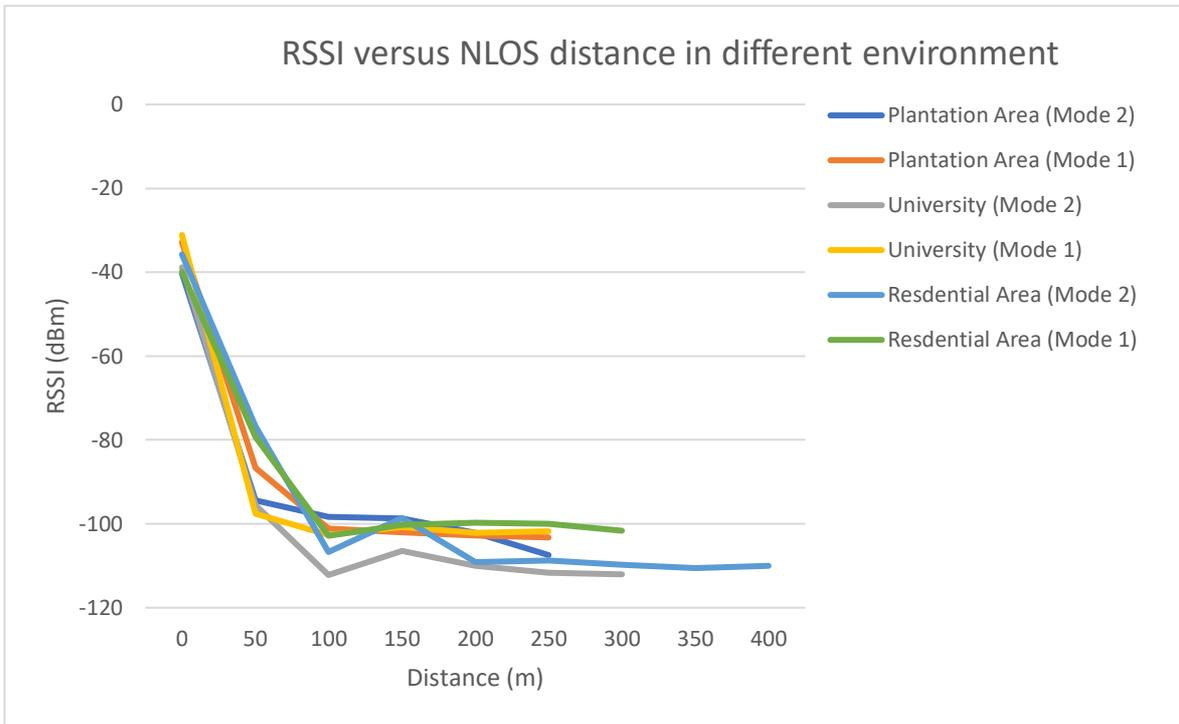
**Figure 11.** The graph for RSSI versus NLOS distance sensors in different environments
