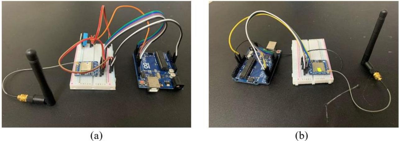
**Figure 2.** (a) Setup for transmitter sensor node, (b) Setup for receiver node
