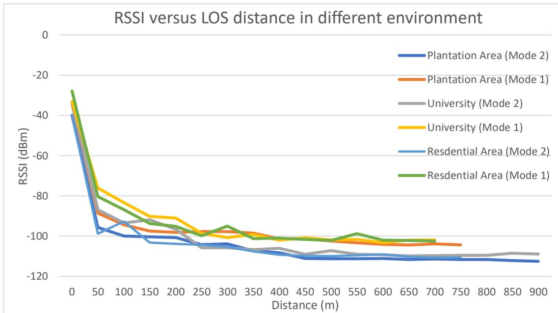
**Figure 9.** The graph for RSSI versus LOS distance sensors in different environments
