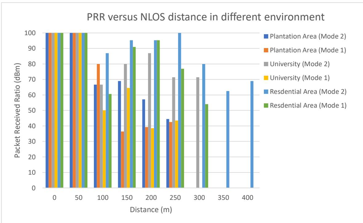
**Figure 12.** The graph for PRR versus NLOS distance sensors in different environments
