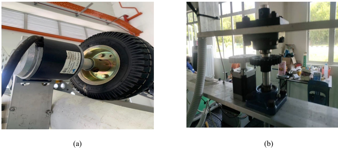
Figure 4 (a) DC motor model XYD-6D (b) Stepper motor
