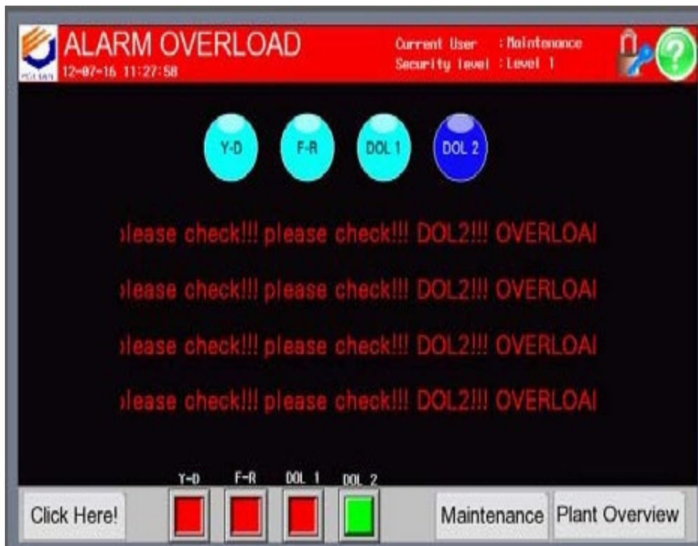
Figure 13. Testing the Overload Alarm Page
