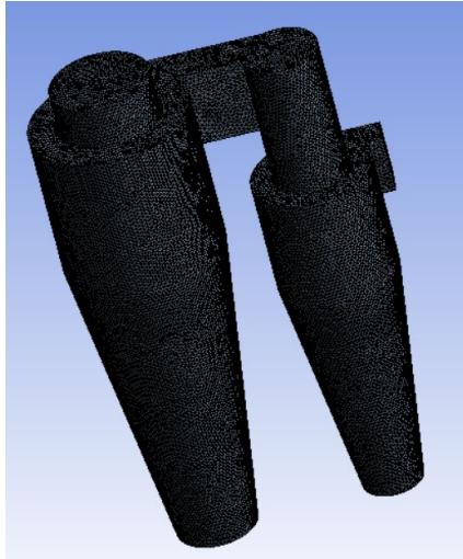
Figure 3. Mesh of cyclone separators with 769907 elements
