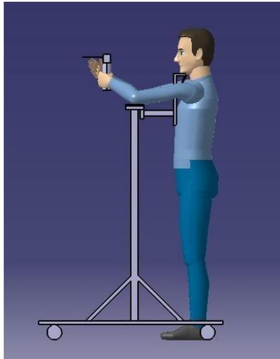
**Figure 9:** Side view of welding assembly tool
