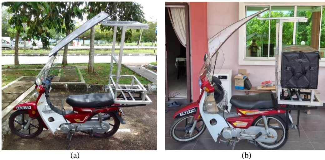
Figure 7. Roof assembly on two different motorcycle brand: (a) AVETA DY90 and (b) DEMAK EX90
