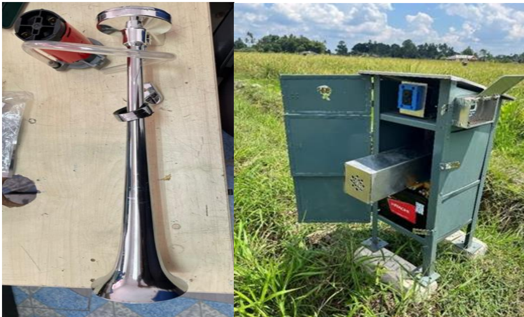
Figure 5. Internal parts of air horn device and Field test setup
