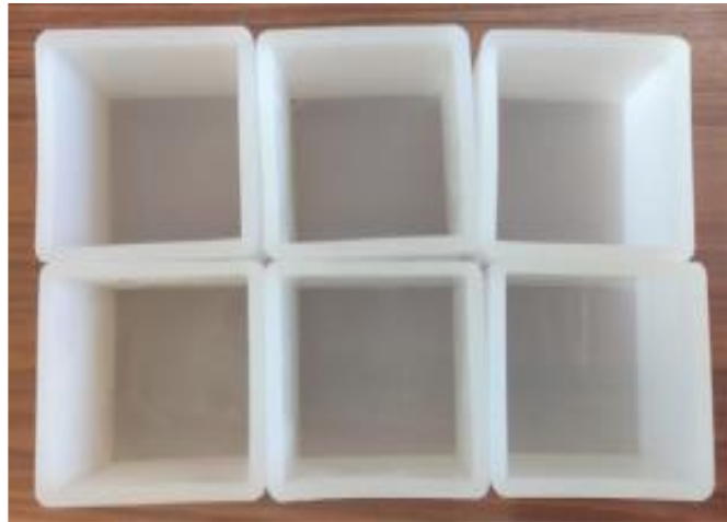
Figure 3. 5 cm x 5 cm Silicone Cube Mould
