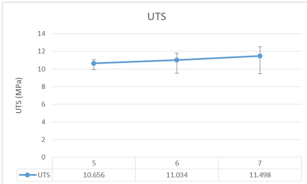
Figure 5. The effect of pressure to Ultimate Tensile Stress
