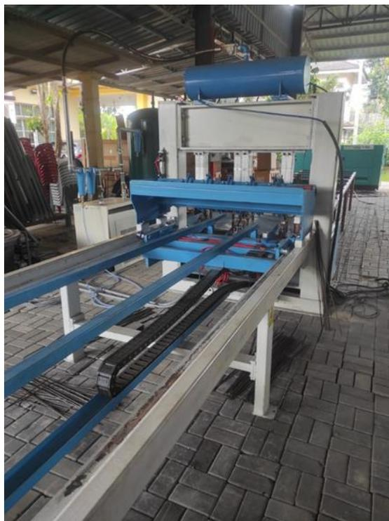
**Figure 1.** Welding-bending machine
