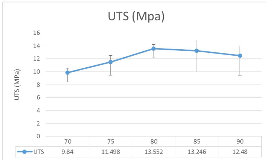
**Figure 3.** The effect of current to Ultimate Tensile Stress
