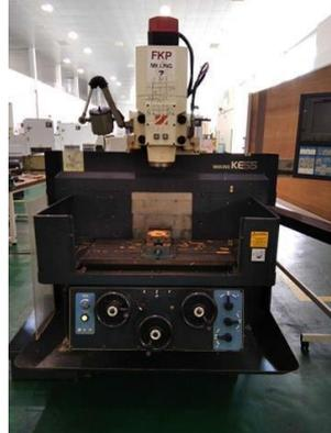
**Figure 6:** NC milling machine (MAKINO KE55)
