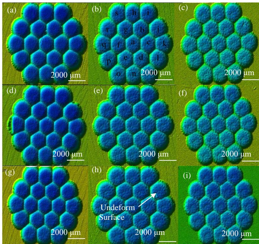
**Figure 6.** 3D Topography of Micro Dimple using Copper Electrode under 3D Laser Microscope
