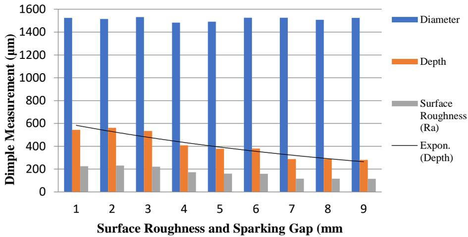
**Figure 10.** Dimple Measurement (Diameter, Depth and Surface Roughness,  $R_a$ ) with Respect to Surface Roughness and Sparking Gap (Copper Electrode)
