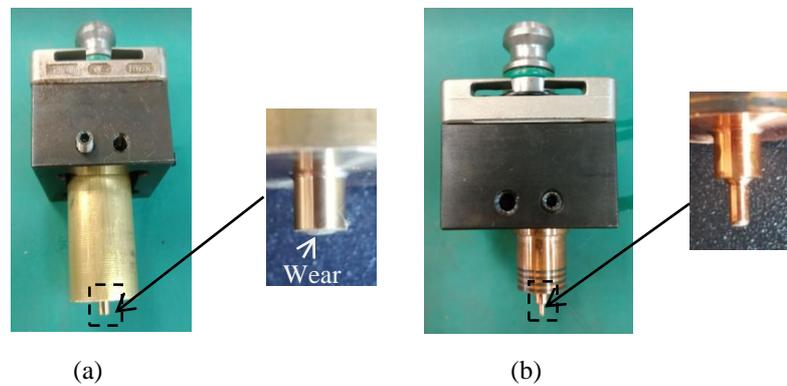
**Figure 11.** Tool Electrode Conditions (a) Magnified View of Brass Electrode (b) Magnified of Copper Electrode
