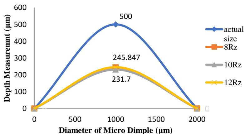
**Figure 7.** Depth Measurement with Respect to Surface Roughness (Brass Electrode)
