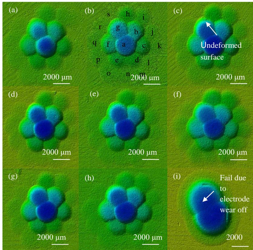
**Figure 5.** 3D Topography of Micro Dimple using Brass Electrode under 3D Laser Microscope
