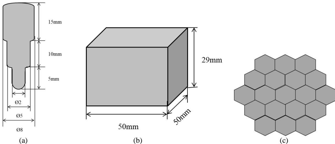
**Figure 1.** Schematic Diagram of the (a) Tool Electrode Design, (b) Workpiece, and (c) Micro dimple
