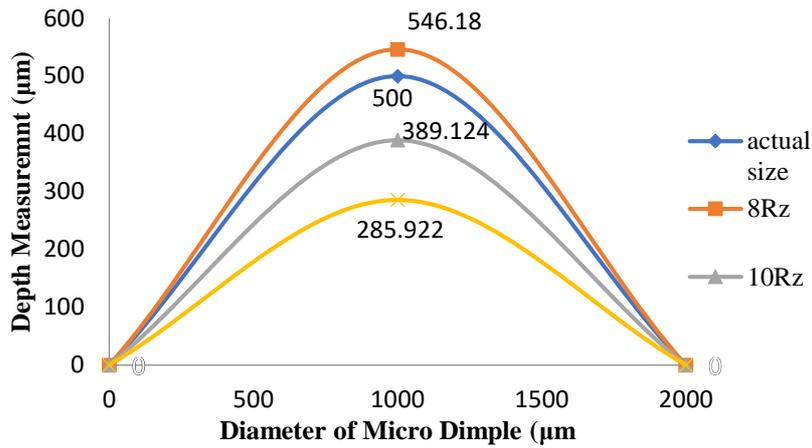
**Figure 8.** Depth Measurement with Respect to Surface Roughness (Copper Electrode)
