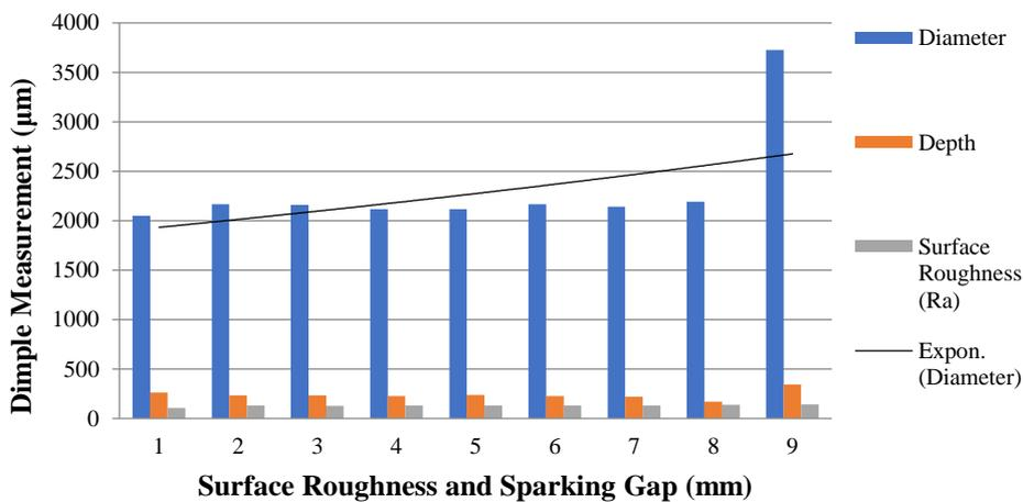
**Figure 9.** Dimple Measurement (Diameter, Depth and Surface Roughness,  $R_a$ ) with Respect to Surface Roughness and Sparking Gap (Brass Electrode)
