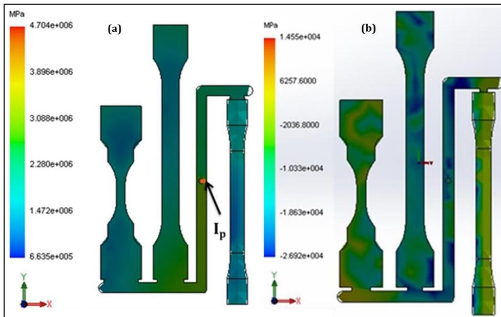
**Figure 8.** Residual stresses of actual (a) and new proposed (b) gate size system.
