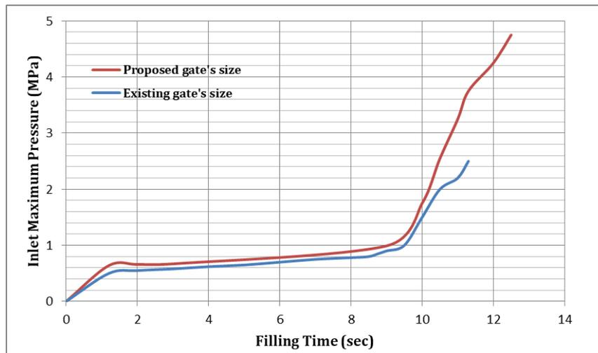
**Figure 9.** Inlet injection pressure as a function of filling time.
