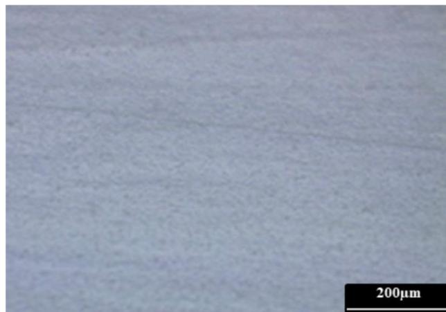
**Figure 3.** Flawless surface for the optimal injection parameters.
