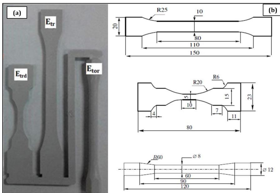
**Figure 1.** The obtained specimens (a) and their dimensions(b) in mm.
