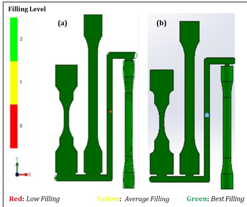
**Figure 5.** Easy filling of actual (a) and new proposed (b) gate size system.
