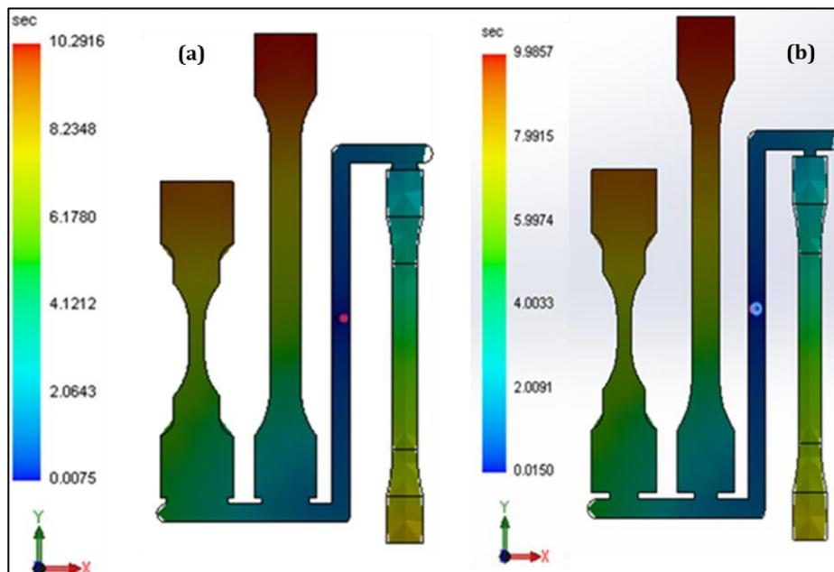
**Figure 6.** Filling time of actual (a) and new proposed (b) gate size system.
