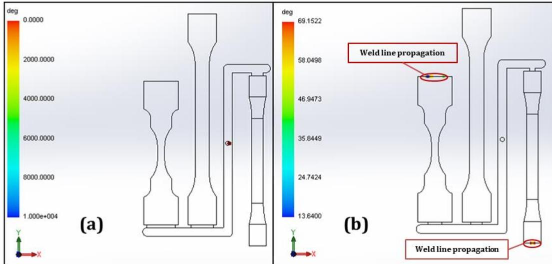
**Figure 7.** Weld line propagation of actual (a) and new proposed (b) gate size system.
