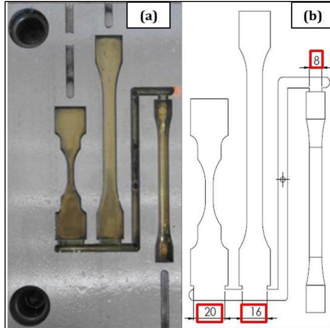
**Figure 2.** The injection mold (a) and the actual gate size in mm (b).
