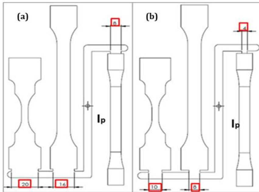
**Figure 4.** The actual (a) and the proposed (b) gate size modification in mm.
