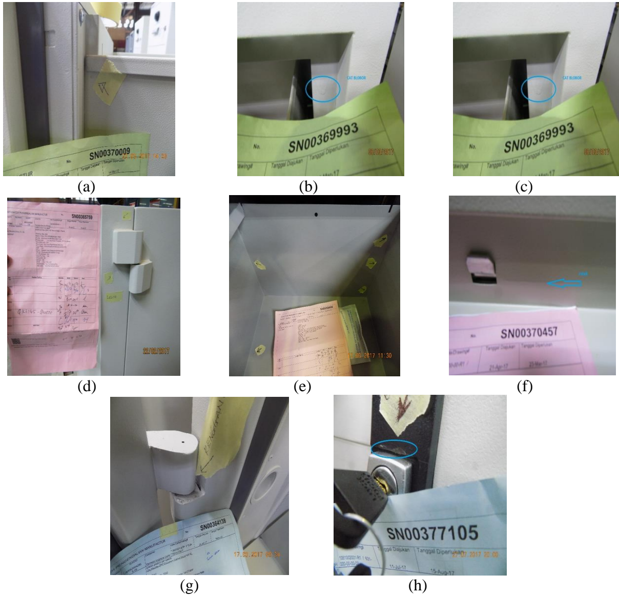
Figure 3. Types of defects, (a) Striped (b) Gap defects (c) Blobor defect (d) Cracked putty (e) Sport is not neat (f) Drawer dent (g) Welding does stick (h) Cracked handle.
