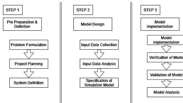
**Figure 3** Model building procedure for production simulation
