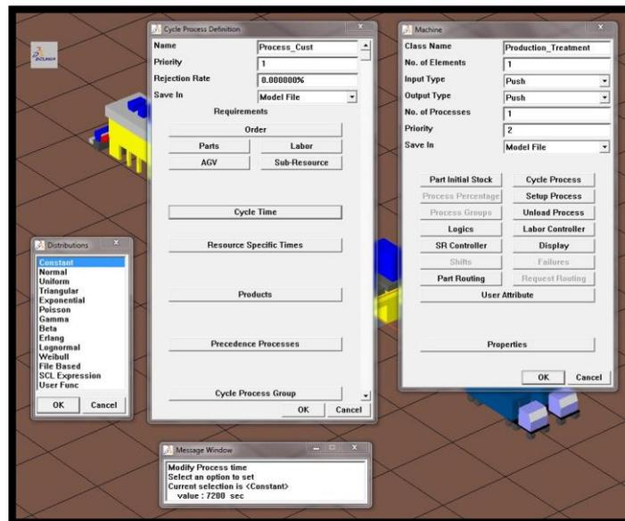
Figure 8 Process cycle time set up in Delmia Quest software
