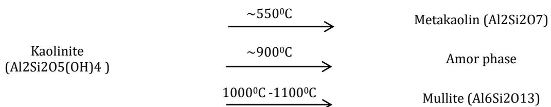
Metakaolin and lime will have reacted well with the presence of hydrated calcium and aluminum silicate [21]. Metakaolin produced from calcination at temperatures of ~ 900 ° C to 1100°C is used in various industries such as paper industry, PVC, wire and cable coating, rubber industry, plastic, adhesive, polishing agent [22].
