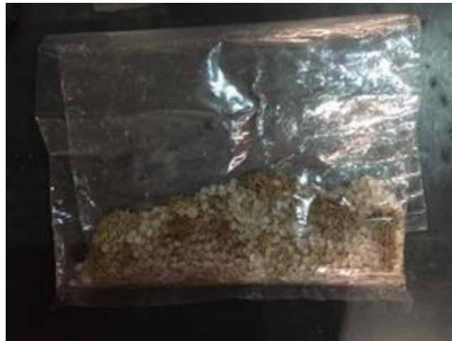
Figure 5 Mixture of EFB fibers, PP and MAPE
