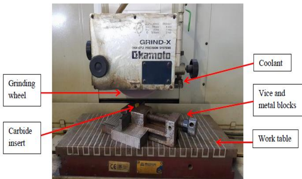
Fig. 1 Surface texturing by grinding process
