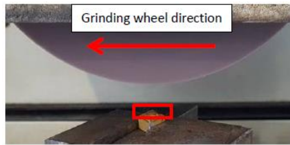
Fig. 2 Parallel grinding direction of wheel to the cutting tip of insert
