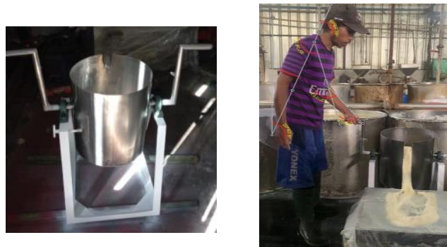
Figure 4. Implementation of the Tofu Pouring Tool
