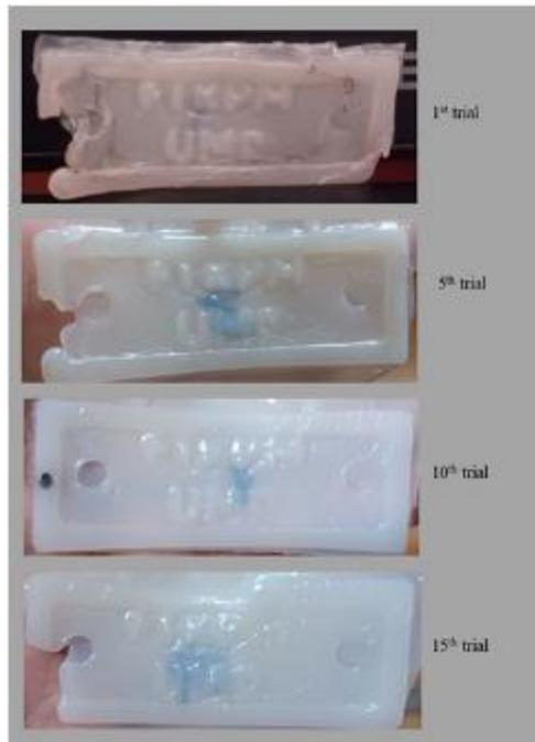
Figure 9. The wording in this keychain specimen is less visible.
