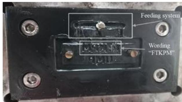
Figure 4. Insert with infill of 75% showing melting area
