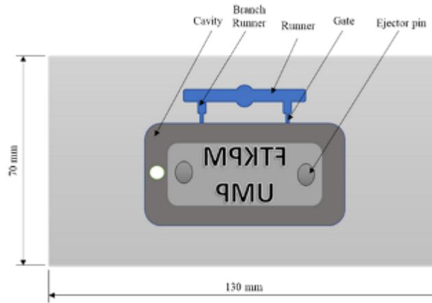
Figure 1. Schematic diagram mold insert.
