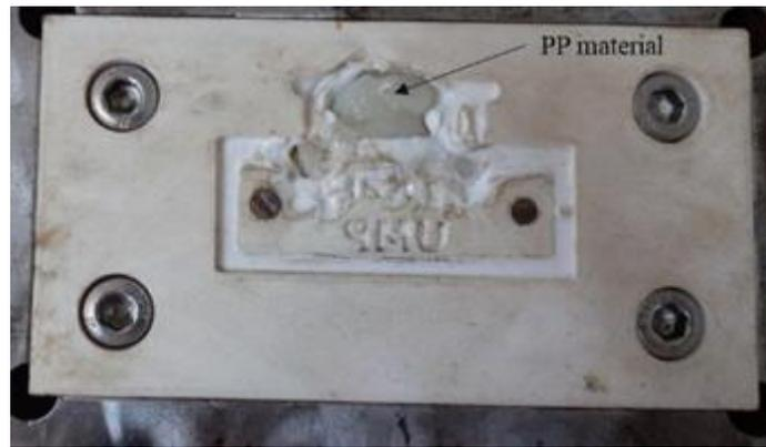
Figure 3. Insert condition after testing (50% infill)
