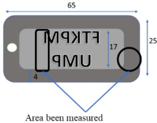
Figure 10. Actual dimension for keychain specimen
