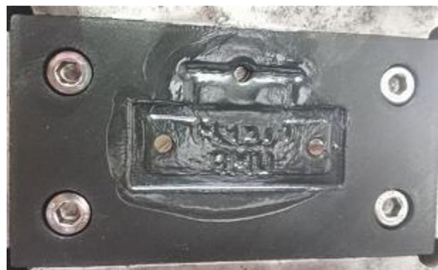
Figure 5. Insert fully melted in cavity area (100% infill)
