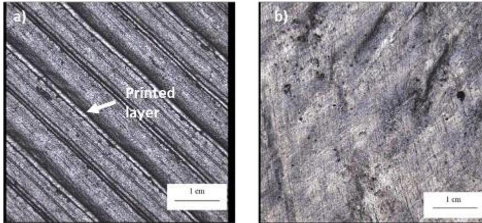
Figure 6. (a) Microstructure image for insert infill 75%, (b) Insert condition under microstructure showing the printed layers after testing.
