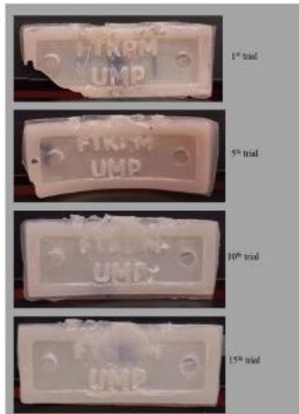
Figure 8. Keychain specimen after injected molten polymer.
