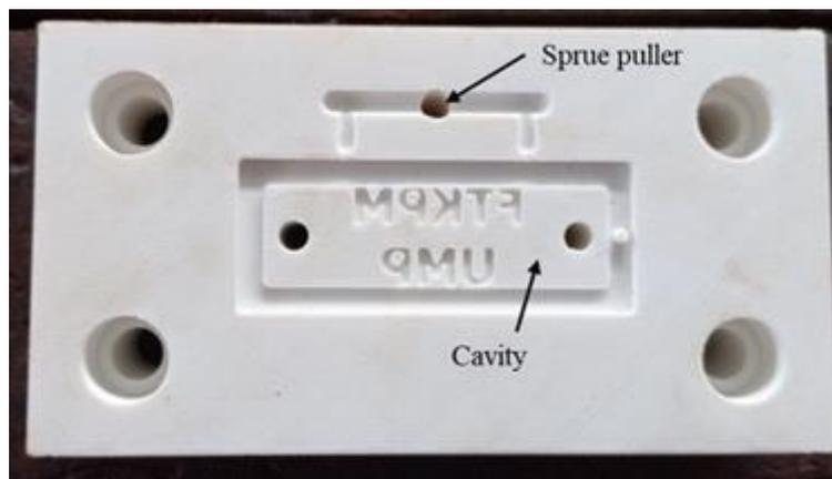
Figure 2. 3D printed mold insert
