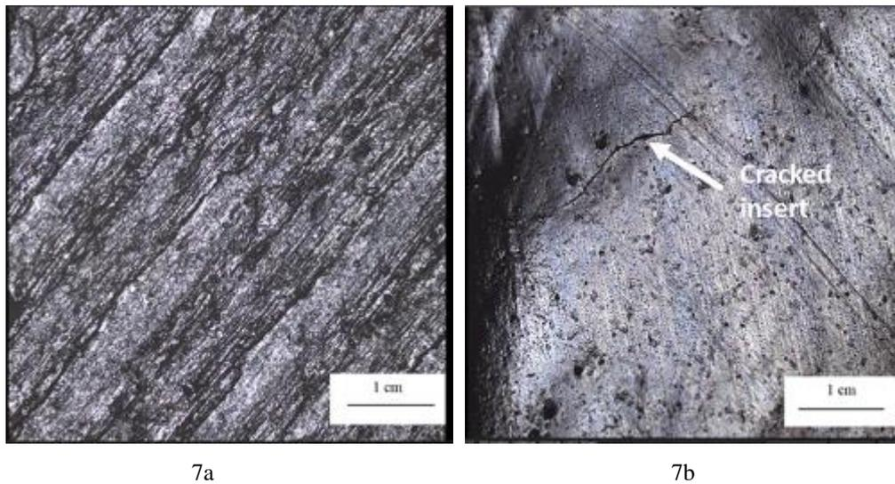
Figure 7. (a) Microstructure image of insert, (b) Image at micro level for insert infill 100% after testing
