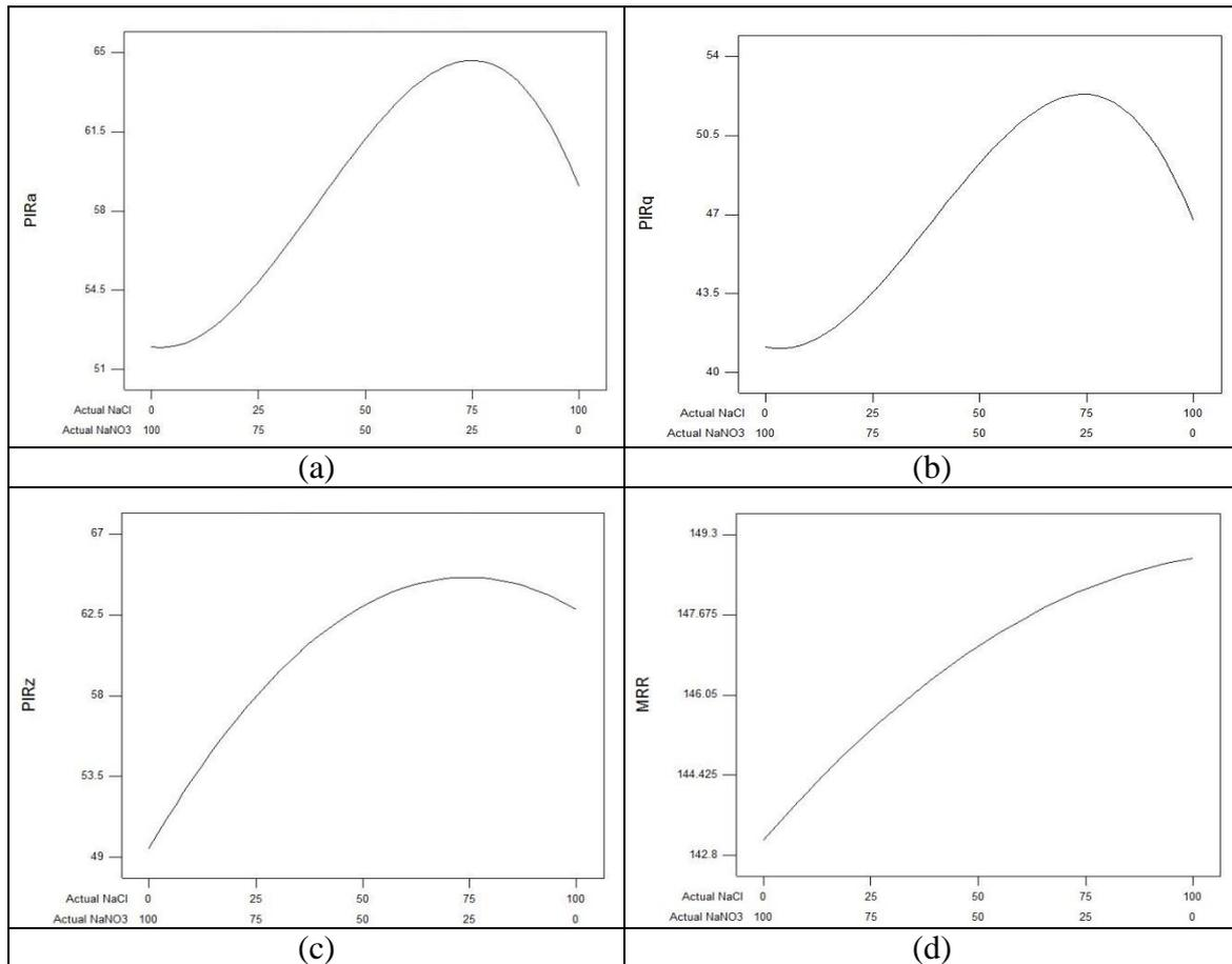
Figure 3. Effect of electrolyte composition on:(a) percentage improvement in average surface roughness; (b)percentage improvement in root mean square surface roughness; (c) percentage improvement in maximum surface roughness; and (d) material removal rate.
