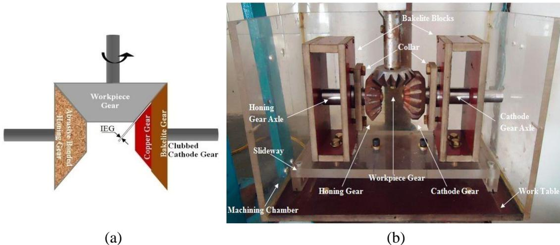
Figure 1.(a) Schematic of principle of ECH process of bevel gears; (b) photographic view of tooling system developed for ECH of bevel gears.
