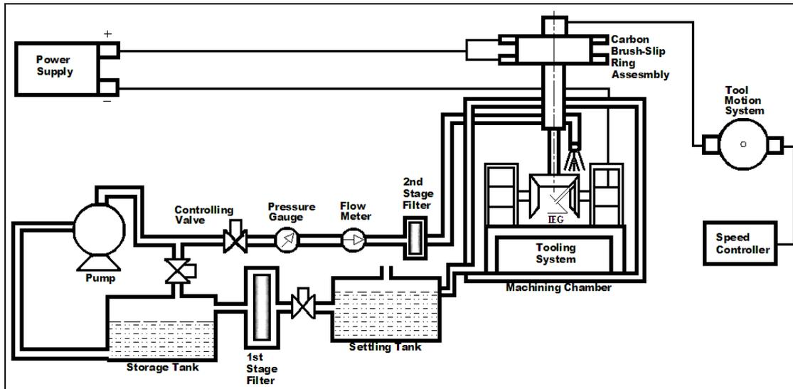
Figure 2. Schematic diagram of experimental setup for ECH of bevel gears.
