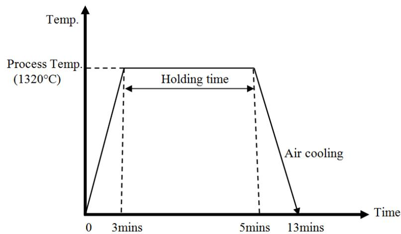
Figure 2. Temperature profile of sample inside the vertical tube furnace.
