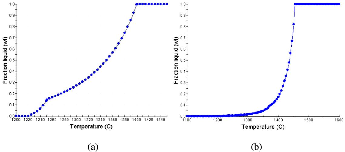
Figure 3. Liquid fraction profile with chemical composition of: (a) AISI D2 tool steel; and (b) AISI 304 stainless steel obtained from JMatPro simulation.
