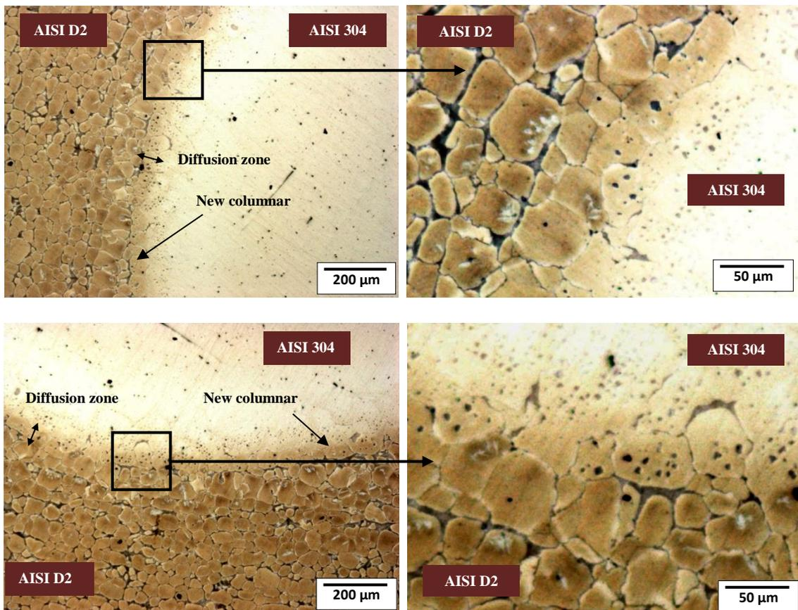
Figure 4. Microstructure of the joint interface of the AISI D2/AISI 304 pair.
