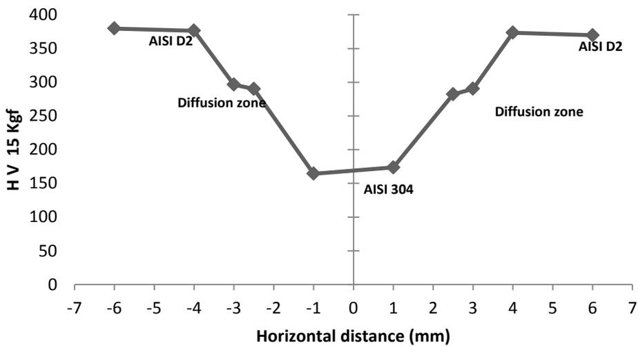
Figure 5. Vickers hardness profile.
