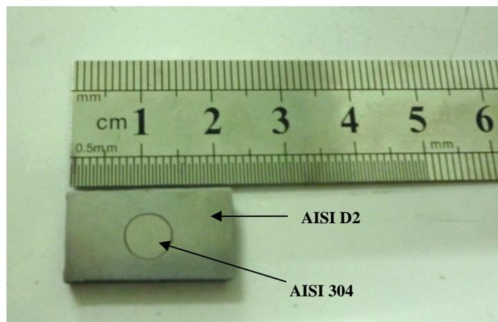
Figure 1. Combination of the two different materials.
