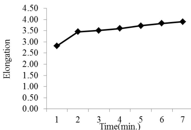
Figure 7. Creep test elongation time (minute)
