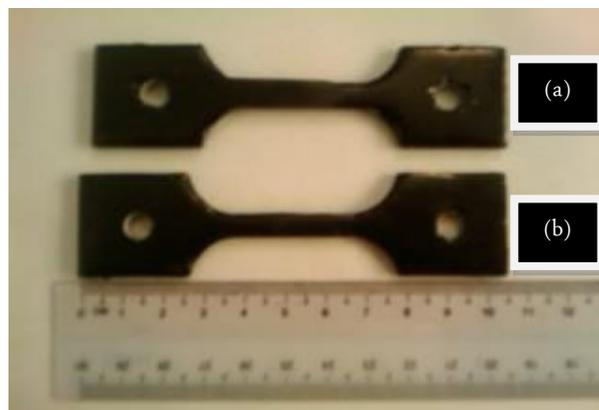
Figure 6. Differences in length of specimens after creep testing.
