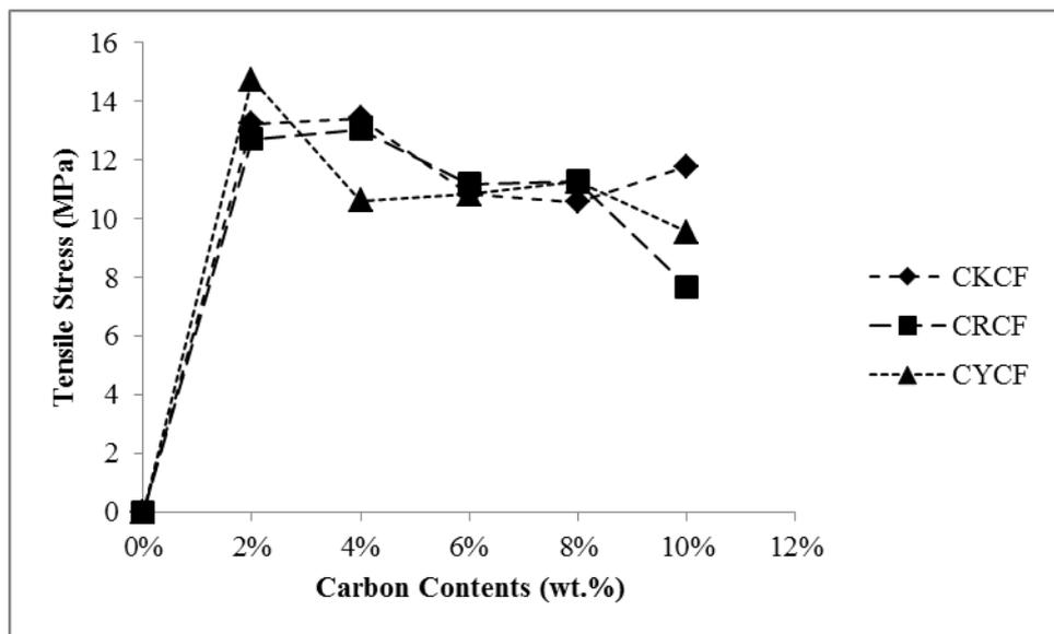
Figure 3. Tensile stress for CKCF, CYCF and CRCF composites.
