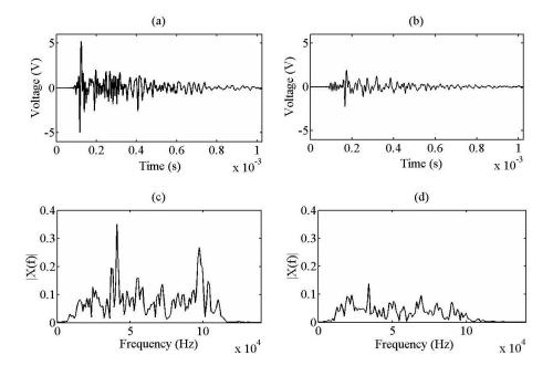
Figure 6.Response due to PLB at point D: (a) and (c) are from sensor '1', while (b) and (d) are from sensor '2'.
