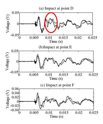
Figure 8.Effect of the low frequency wave traveling across the perforated region (indicated by red circle).Two lines in each figure indicate the two waveforms captured by the two different sensors (sensor '1' and sensor '2').
