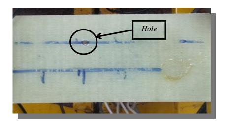
Figure 1. Gl/epoxy resin laminates for the experiments.
