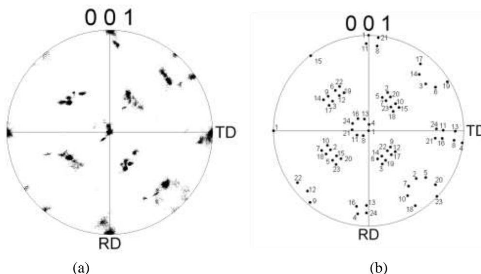
Figure 1. (a) A 001  $\alpha$  pole figure of EBSD analysis data for bainitic ferrite held at 560°C for 1 hour, and (b) Configuration of  $\langle 001 \rangle \alpha$  poles for the K-S variants adjusted to (a).
