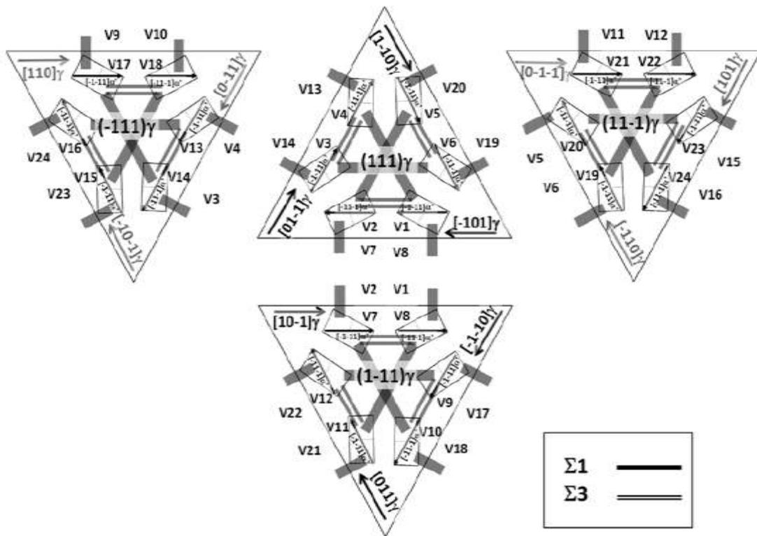
Figure 2. Illustration of the 24 crystallographic variants (V1-V24) evolving in the  $\{111\}$  austenite plane in the K-S orientation relationship. The triangles and rectangles indicate the  $\{111\}$  austenite (FCC) plane and  $(011)$  martensite (BCC) plane respectively [10].
