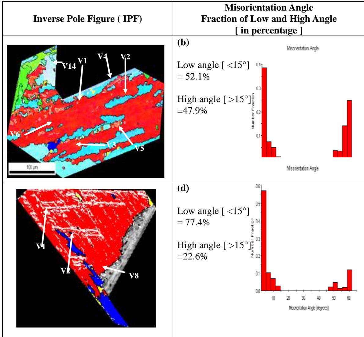
Figure 5. Variant determination and distribution of low angle and high angle misorientation in each condition: (a), (b) 560 °C, (c), (d) 580 °C.
