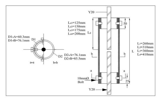
Figure 1. Detailing of grouted splice sleeve connector.
