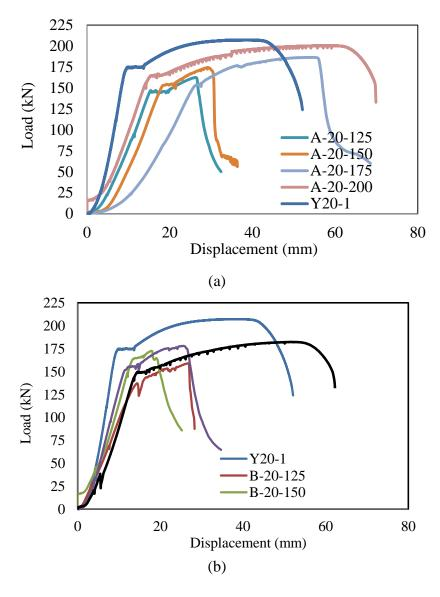
Figure 4. Load-displacement graph of connectors: (a) Type A; (b) Type B.
