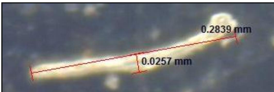
Figure 1. Dimension of the pulverised kenaf bast fibre.
