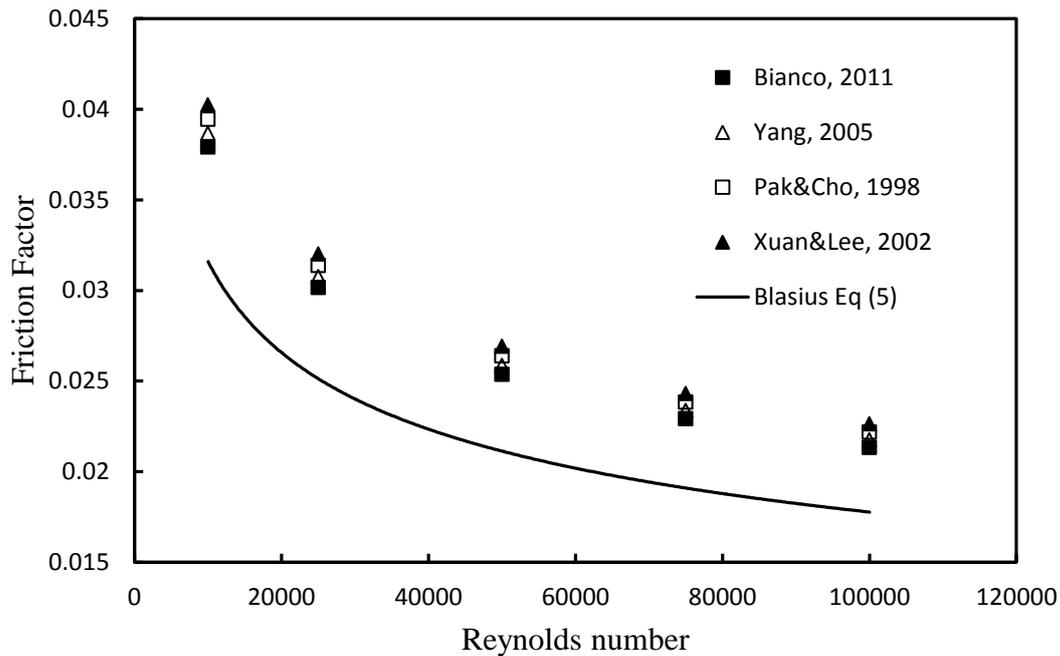
Figure 3. Friction factor at different Reynolds number.
