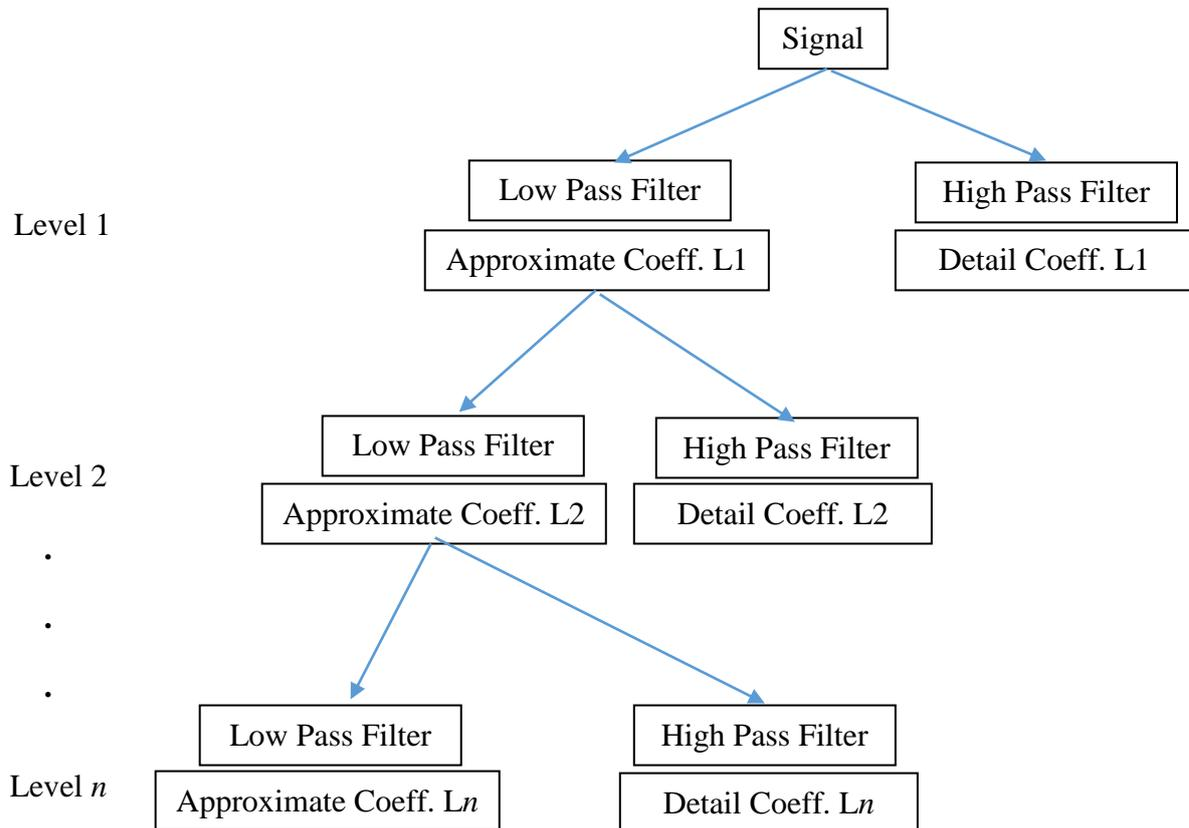
Figure 2. Discrete wavelet transform.
