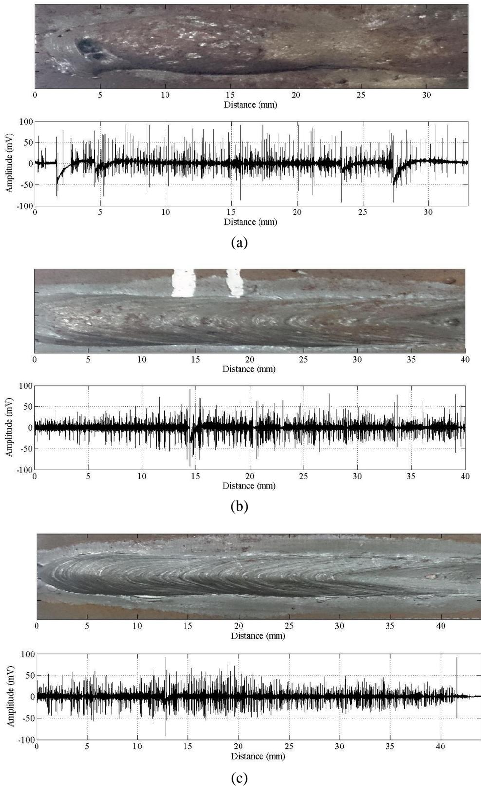
Figure 3. The acquired sound signal during welding process
