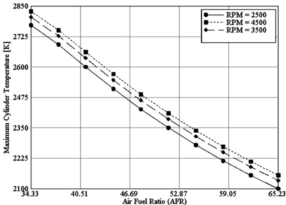
Figure 5. Variation of maximum cylinder temperature vs. AFR.
