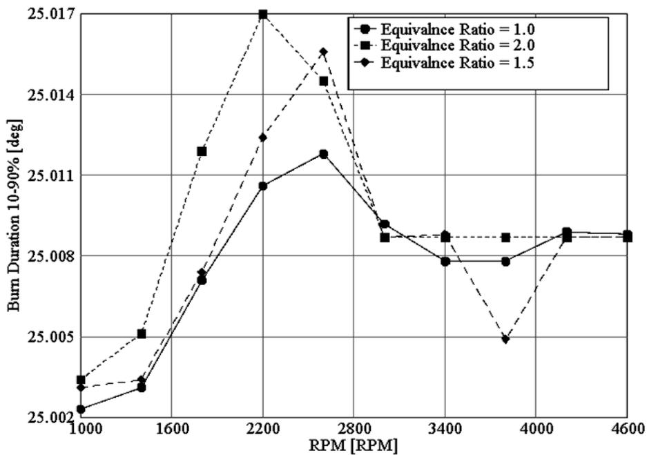
Figure 7. Combustion duration vs. RPM.
