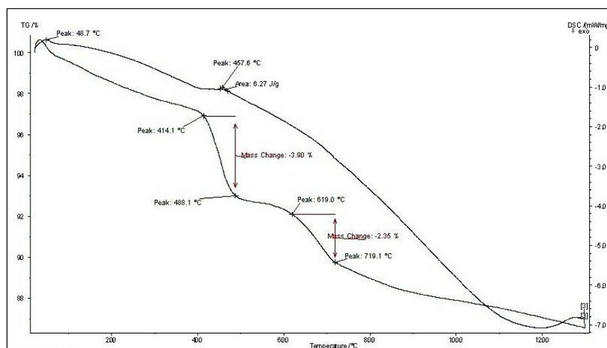
Figure 1. DSC/TG Curves for As-Prepared Powder S100
