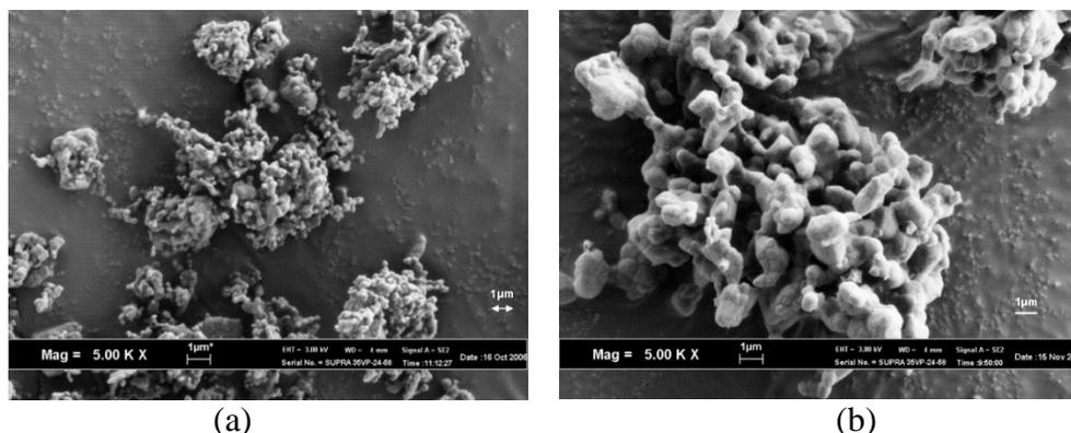
Figure 4. Morphology by FESEM of S200 powders calcined for 1 hour at (a) 900 °C and (b) 1000 °C
