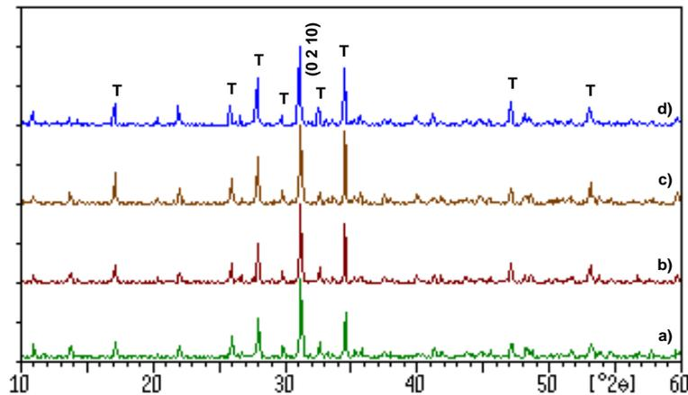
Figure 3. XRD patterns of S200 powder calcined at 900°C for different soaking durations [All peaks are assigned to  $\beta$ -TCP] a) 1 hour, b) 2 hours, c) 3 hours and d) 4 hours.
