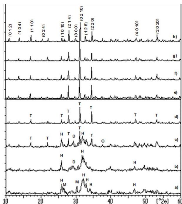
Figure 2. XRD patterns of S200 powders before and after calcination at different temperatures for 2 hours soaking (a) as-prepared powder, (b)  $500^\circ\text{C}$ , (c)  $700^\circ\text{C}$ , (d)  $900^\circ\text{C}$ , (e)  $1000^\circ\text{C}$ , (f)  $1100^\circ\text{C}$ , (g)  $1200^\circ\text{C}$ , and (h)  $1300^\circ\text{C}$ . [H – HA; M – Monetite; D –  $\beta$ -DCP; T-  $\beta$ -TCP; O – CaO].
