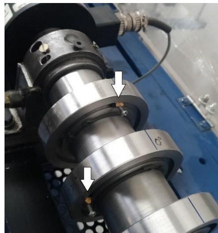
Figure 6. Detail showing dovetail machining where the unbalance masses are installed.
