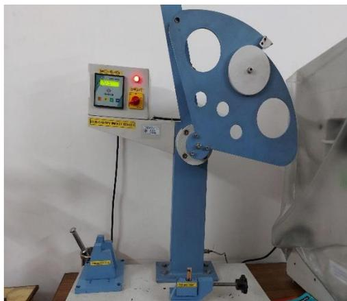
Figure 7. Izod impact test equipment
