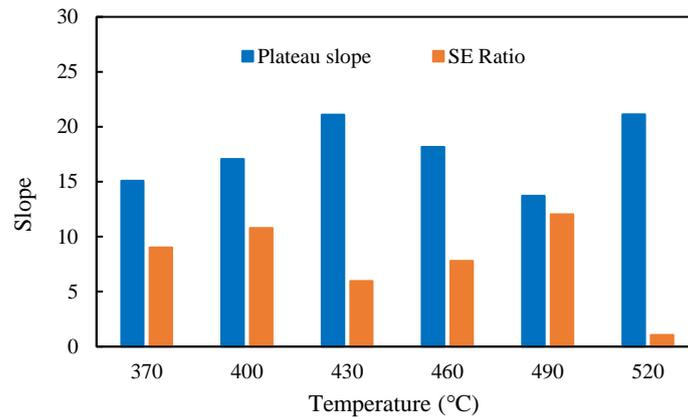
Figure 3. Plateau slope and SE ratio at different heat treatment condition
