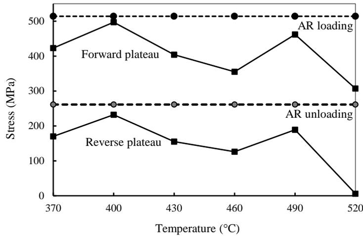
Figure 5. Effect of aging temperature on stress induced deformation for NiTi alloy aged for 15 minutes
