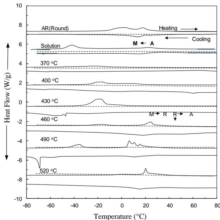
Figure 6. Thermal transformation behavior of the NiTi superelastic alloy after ageing for 15 minutes at various temperatures
