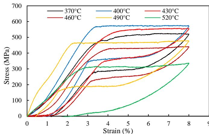
Figure 4. NiTi wire's stress-strain superelastic response at temperatures between 370 and 520 °C for 15 minutes
