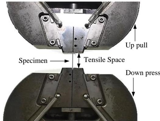
Figure 2. ISO standard 6892 NiTi archwire tensile deformation setup
