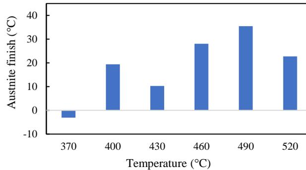
Figure 7. Thermal transformation behavior of the NiTi superelastic alloy after 15 minutes of ageing at various temperatures
