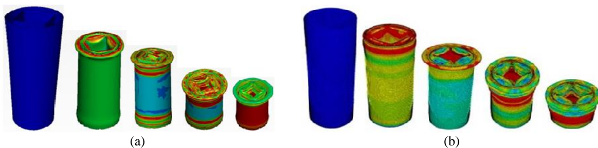
Figure 5. Failure mode of bi-tubes under axial compression obtained by: (a) FEA analysis and (b) Numerical analysis performed by [16]
