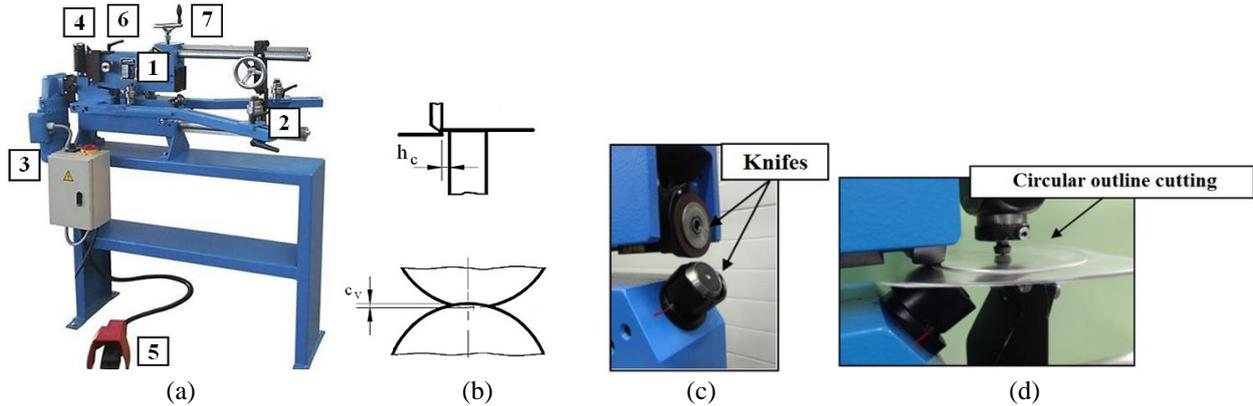
Figure 2. Experimental equipment and main parameters: (a) shear-slitting device: 1 – cutting tools, 2 – sheet holder, 3 – engine, 4 – clearance knob with scale, 5 – drive pedal, 6 – cutting speed knob with scale, 7 – knife overlap regulator (b) main slitting parameters, (c) zoom of cutting tools and (d) example process of circular outline cutting
