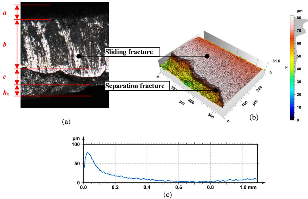
Figure 4. Sheared edge characteristic features and its measurement: (a) image of the cut surface, (b) geometric structure of the cut surface and (c) profile of bottom sheet surface with visible burr area
