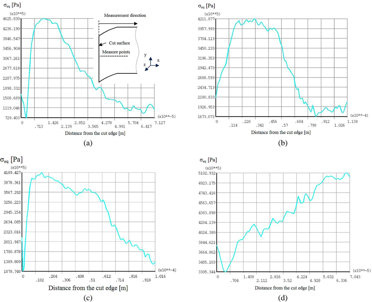
Figure 17. Influence of cutting clearance on Huber-Mises equivalent stress values in the area of the cut edge for: (a)  $h_c = 0.03$  mm, (b)  $h_c = 0.09$  mm, (c)  $h_c = 0.15$  mm and (d)  $h_c = 0.21$  mm
