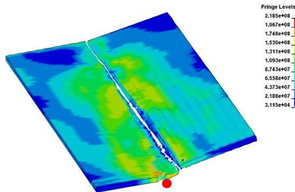
Figure 14. Huber-Mises equivalent stress [Pa] distribution after the cutting process ( $h_c = 0.06$  mm)
