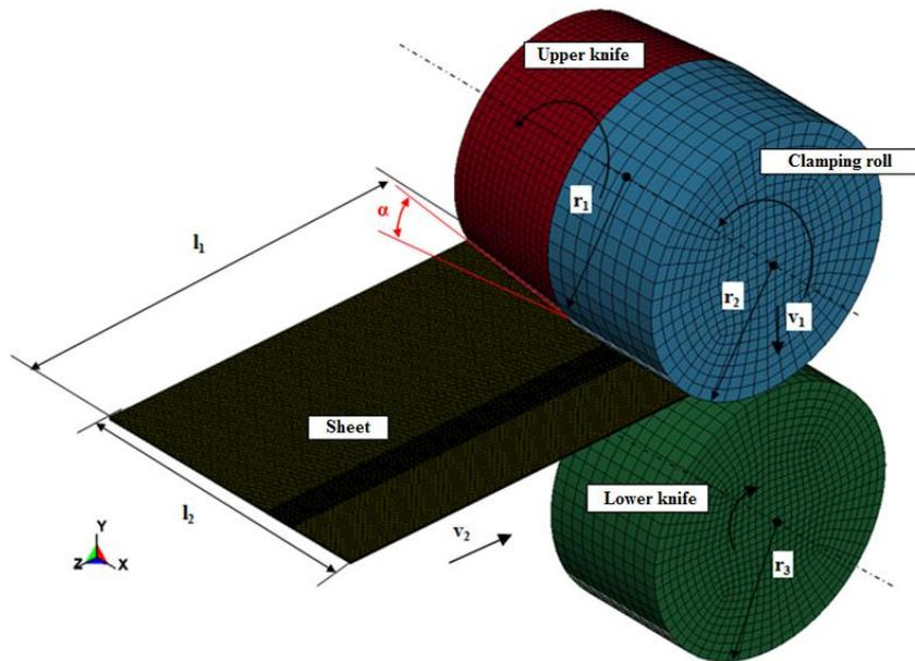
Figure 12. FEM model of the shear-slitting process
