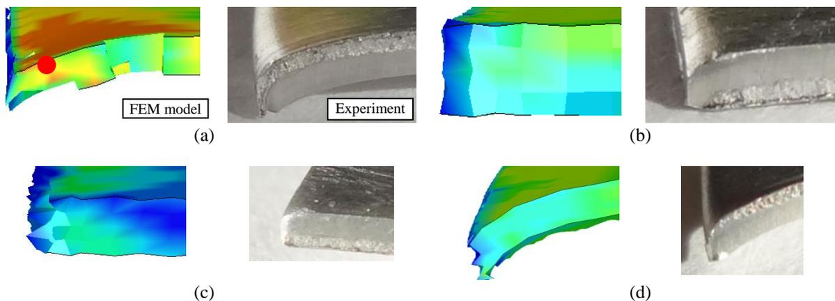
Figure 15. An exemplary comparison of the bends of the cut surfaces obtained as a result of the experiment and simulation: (a)  $h_c = 0.06$  mm, (b)  $h_c = 0.09$  mm, (c)  $h_c = 0.12$  mm and (d)  $h_c = 0.24$  mm
