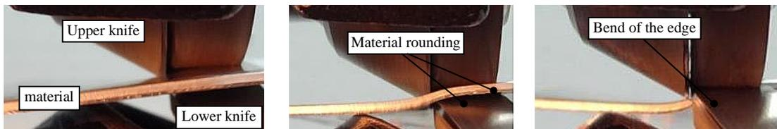
Figure 10. The moment of formation of the bend of the cut surface recorded during the process
