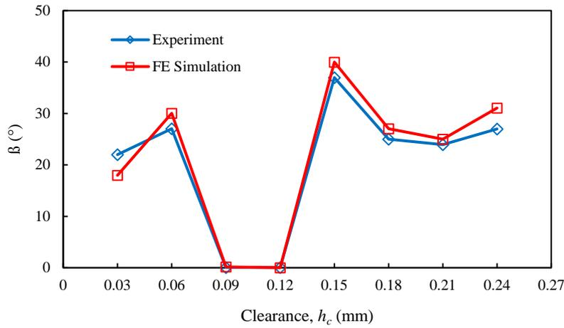
Figure 16. Comparison of the values of the bend angles of the cut surface obtained as a result of the experiment and FEM simulation
