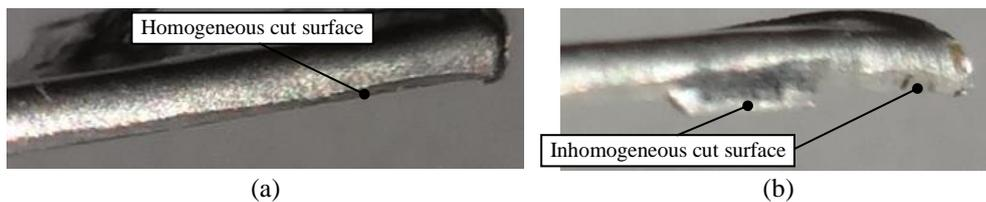
Figure 11. Influence of clearance on the stability of the cutting process in the final stage: (a)  $h_c = 0.12$  mm and (b)  $h_c = 0.15$  mm
