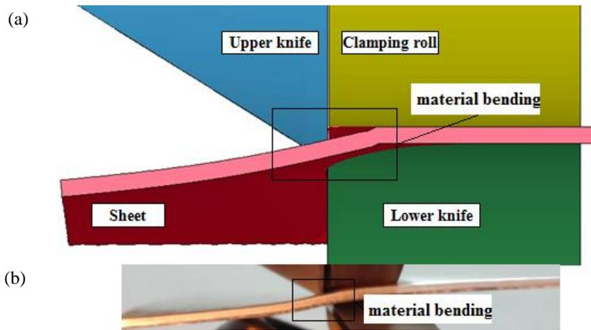
Figure 13. Comparison of the results of the simulation tests with the results of the experiment at the moment of the formation of the bend of the cut surface: (a) simulation model and (b) real process recorded with a camera ( $h_c = 0.06$  mm)
