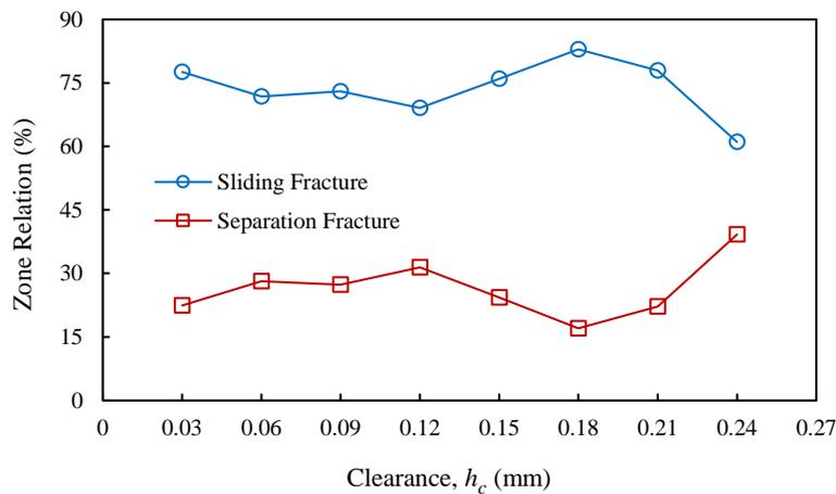
Figure 5. Influence of clearance on formation of sliding and separation fracture
