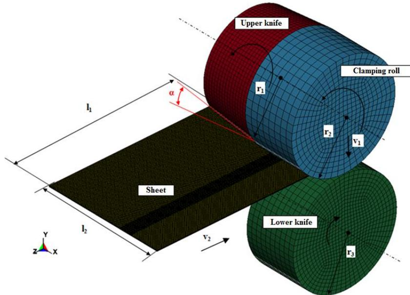
Figure 12. FEM model of the shear-slitting process
