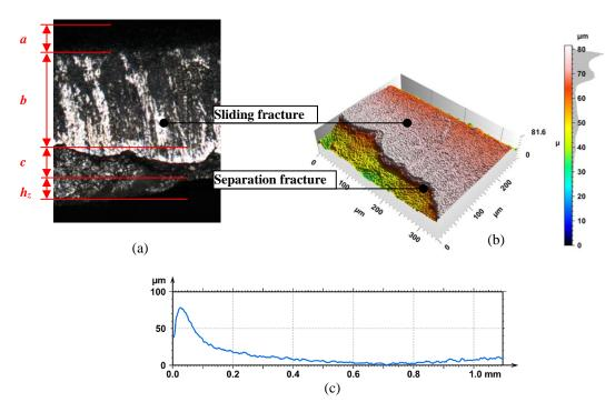
Figure 4. Sheared edge characteristic features and it's measurement: (a) image of the cut surface, (b) geometric structure of the cut surface and (c) profile of bottom sheet surface with visible burr area
