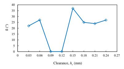
Figure 9. The effect of clearance on the bend angle
