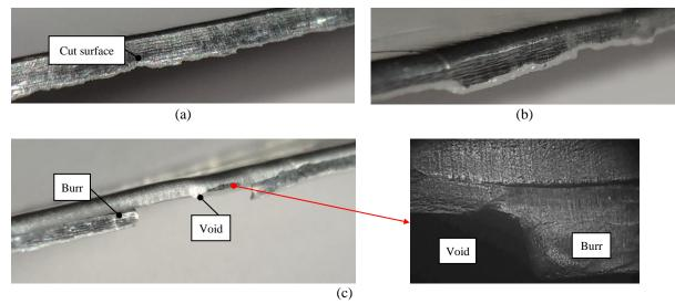
Figure 7. Examples of obtained burrs on the cut surface: (a) regular for  $h_c = 0.03$  mm, (b) irregular  $h_c = 0.06$  mm and (c) irregular leaving a void  $h_c = 0.24$  mm
