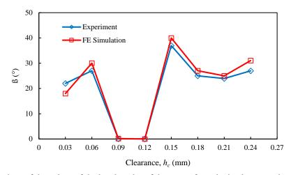
Figure 16. Comparison of the values of the bend angles of the cut surface obtained as a result of the experiment and FEM simulation
