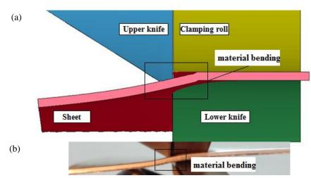
Figure 13. Comparison of the results of the simulation tests with the results of the experiment at the moment of the formation of the bend of the cut surface: (a) simulation model and (b) real process recorded with a camera  $(h_c = 0.06 \text{ mm})$
