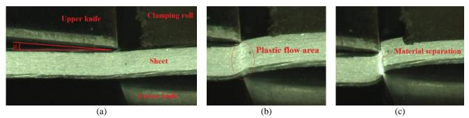
Figure 3. Main shear-slitting phases: (a) elasto-plastic, (b) plastic flow and (c) fracture
