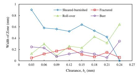
Figure 6. Influence of clearance on the formation of zones on the cut surface
