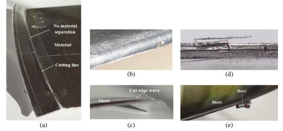
Figure 1. Defects of cut edge of aluminum alloys: (a) no material separation, (b) edge rounding, (c) edge wave, (d) chip and (e) burr
