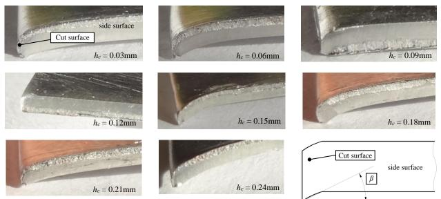
Figure 8. The effect of clearance on the bend of the edge of the cut surface
