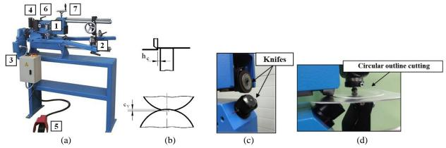
Figure 2. Experimental equipment and main parameters: (a) shear-slitting device: 1 – cutting tools, 2 – sheet holder, 3 - engine, 4 - clearance knob with scale, 5 - drive pedal, 6 - cutting speed knob with scale, 7 - knife overlap regulator (b) main slitting parameters, (c) zoom of cutting tools and (d) example process of circular outline cutting
