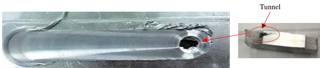
Figure 8. Tunnel defect in the middle of the overlapped welded piece
