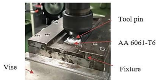
Figure 3. Fixture clamp during joining FSW
