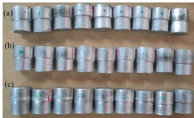
Figure 6. Samples after the extrusion at: (a) 10°, (b) 20° and (c) 30° die angles
