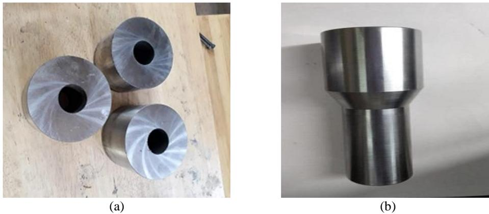
Figure 3. Individual parts before the extrusion process: (a) dies and (b) punch
